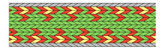
"Dotted" pattern. 12 tablets are turned all together continuously in one direction. The same pattern, but running in the opposite direction, is repeated on the back side of the belt.
